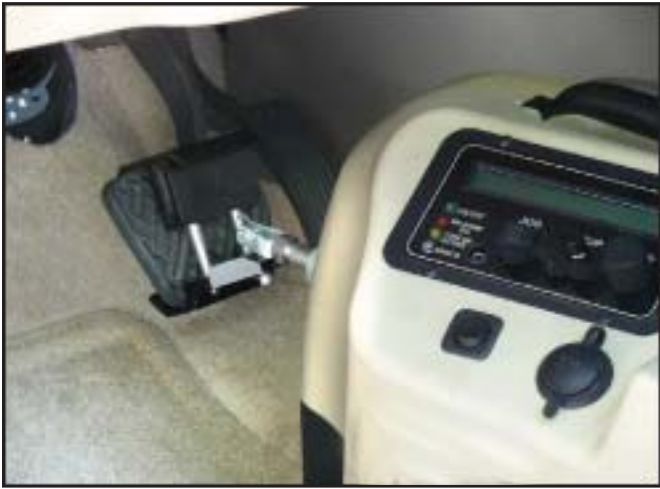
Fig. 1 Place clamp on brake pedal
