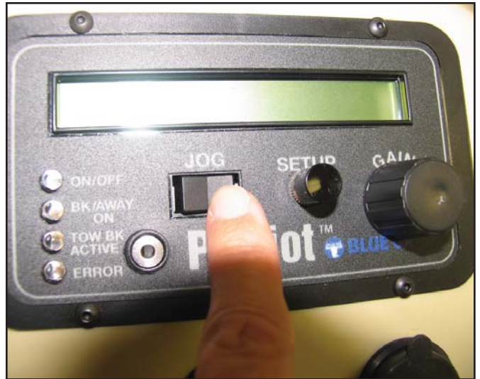
Fig. 3 Adjust the brake pedal with the Jog Switch
