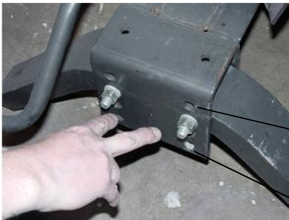
Figure 1-Determining Side Frame mounting bolts location
