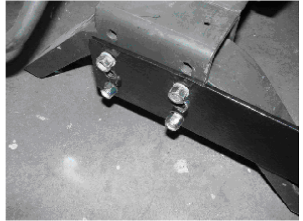
Figure 4-Left Side Plate attached
